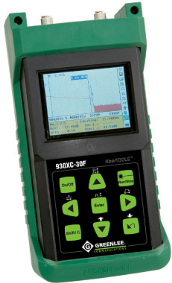
Figure 3. An OTDR measures the length to a fault or the length of singlemode and multimode fiber-optic cables.
