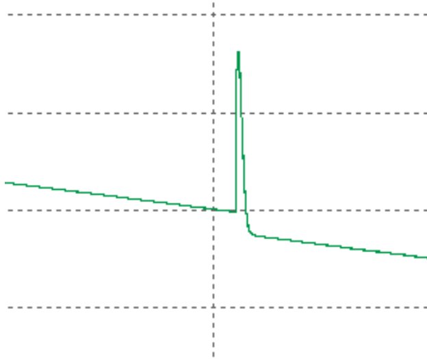
Figure 4. Example OTDR image of a lossy connector (IL = 1.09 dB; RL = -35.7 dB). Figure 4. Example OTDR image of a lossy connector (IL = 1.09 dB; RL = -35.7 dB).
