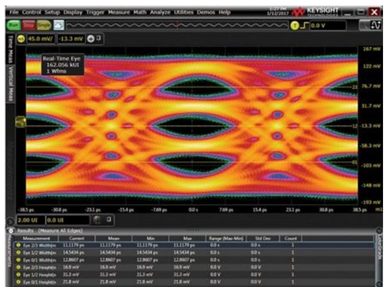
FIGURE 1. Example PAM4 eye diagram showing the four encoding states. (Photo courtesy of Keysight Technologies)
